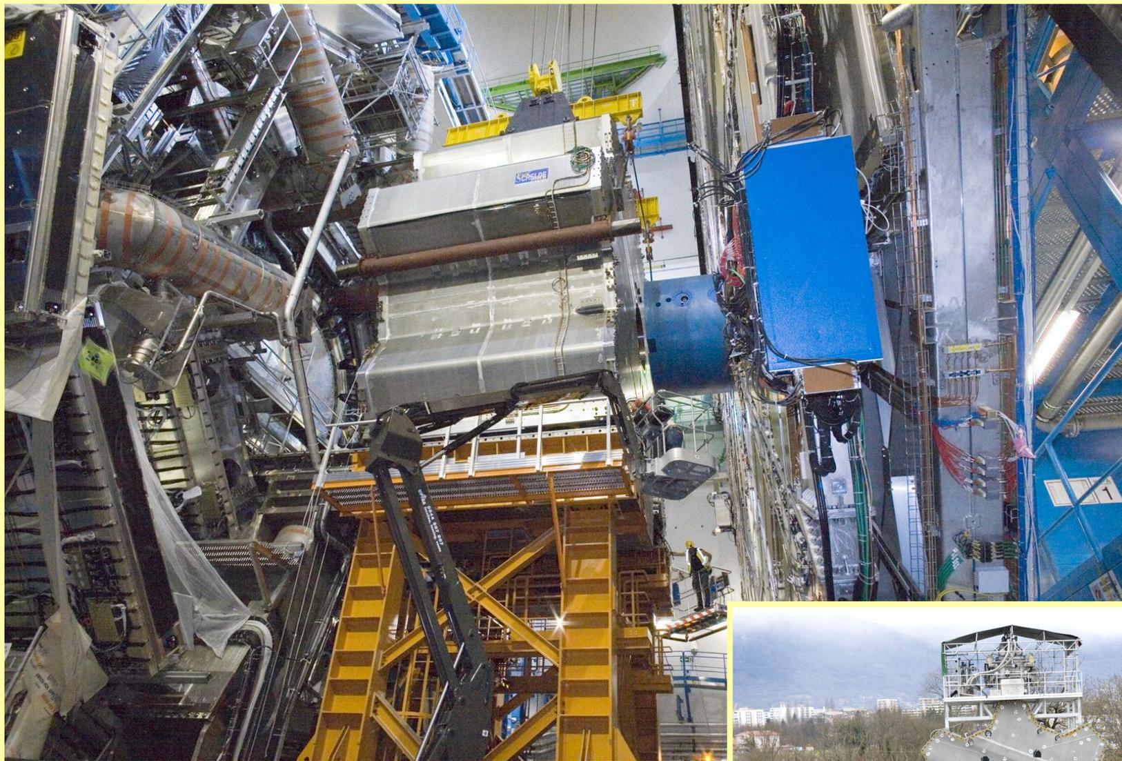
The two end-cap toroid magnets
