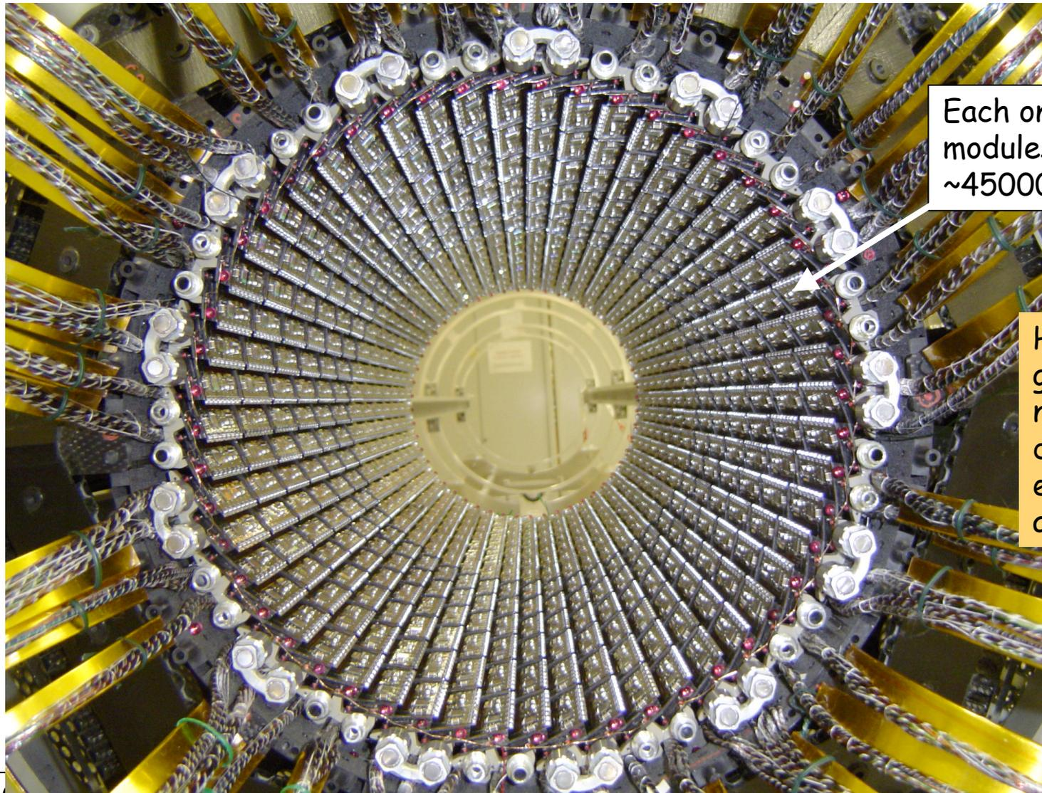
Each one of these modules contains  $\sim 45000$  pixel sensors
