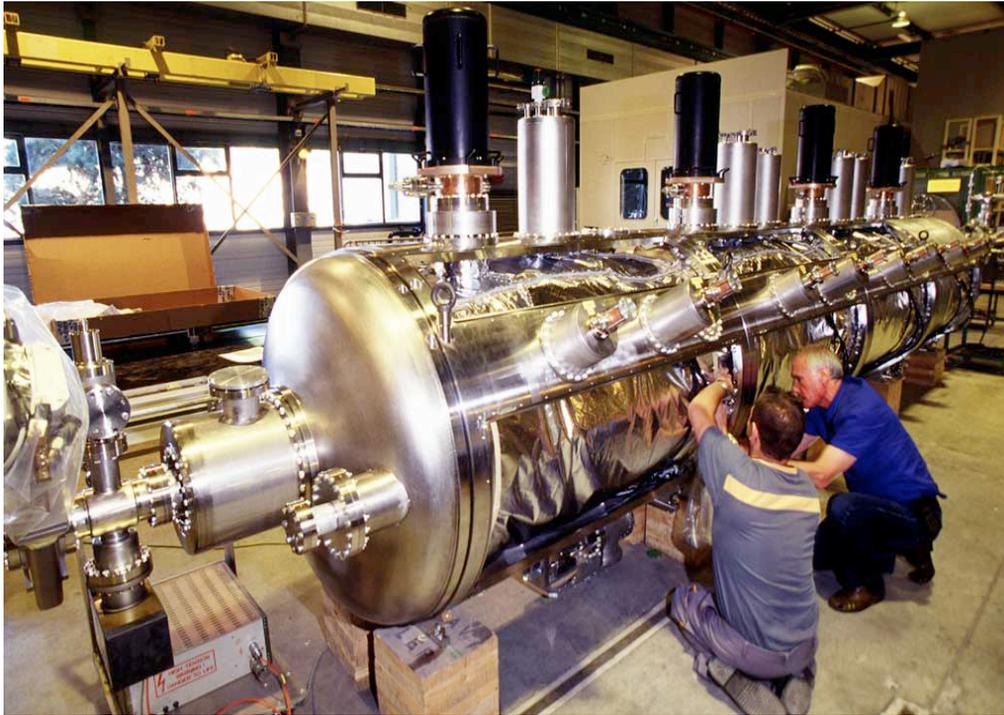
The LHC uses 8 superconducting cavities per beam, delivering 16 MV (an accelerating field of 5 MV/m) at 400 MHz.
