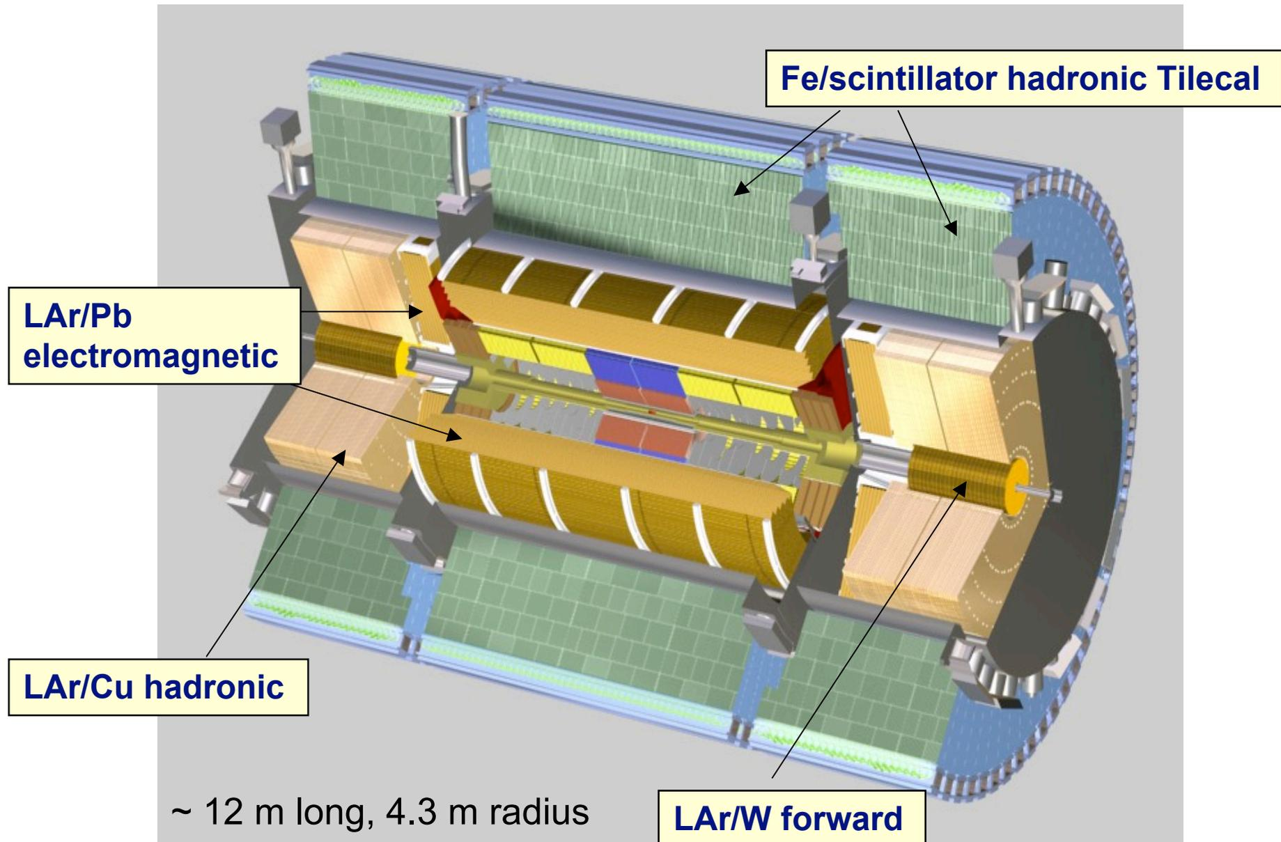
Barrel calorimeter (EM Pb/LAr + Hadron Fe/scintillator) in its final position at Z=0. EM calorimeter is filled with LAr and cold (87 K)
