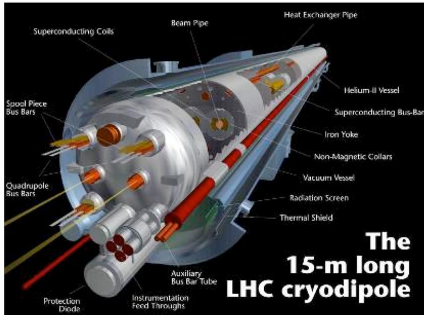
The LHC most challenging components are 1232 high-tech superconducting dipole magnets
