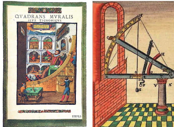
Fig. Pref.1b Two measurement devices used by Tycho Brahe. On the left a wall quadrant in the Uraniborg observatory on the island of Hven (or Ven) located between Denmark and the southern Swedish province of Scania. On the right, Tycho's oversized sextant. Source: Wikipedia article (in French) about Tycho Brahe.
