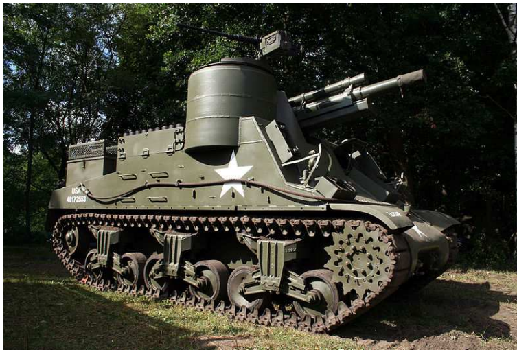
Fig. 6.4 M7 tank. Several versions of the M7 tank were used by the US Army in World War II. For the kind of operation performed in South Korea before the outbreak of the Korean War it was the machine gun at the top (rather than the howitzer) which was the most useful. Source: Wikipedia article entitled “M7 priest”
