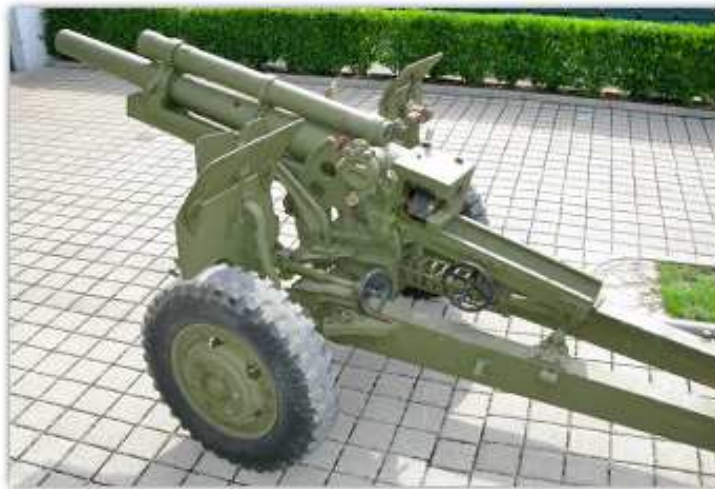
Fig. 6.7 105-mm howitzer. A howitzer is a gun which fires shells at fairly steep angles. It is intermediate between a gun which has high velocity and relatively flat trajectories and a mortar which fires at very steep angles. In almost horizontal position the 105-mm can be used for direct hits with a range of about 1 km. In a steep position, i.e. when really used as a howitzer, the range is about 3 km. Between July and October 1948 a few battalions of the Korean Constabulary received training in the use of machine guns, 57-mm anti-tank guns and 105-mm howitzers. Source: http://www.asphm.com
