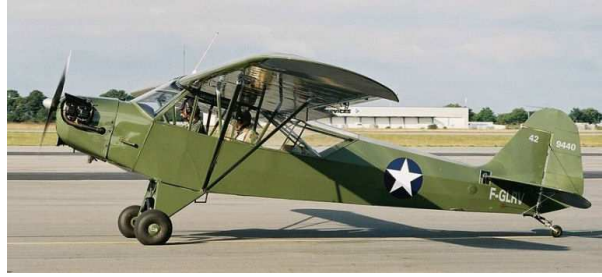
Fig. 6.13 Piper L-4 Grasshopper. The Piper L-1 to L-5 were military versions of the Piper Cub. The designation “L” means Liaison aircraft.
