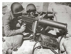
Fig. 2.2 Water cooled machine gun. The picture shows a 0.30 inch water-cooled machine gun which was used in World War II. There was also a similar air-cooled 0.30 machine gun. Source: http://www.rt66.com/korteng/SmallArms/30calhv.htm
