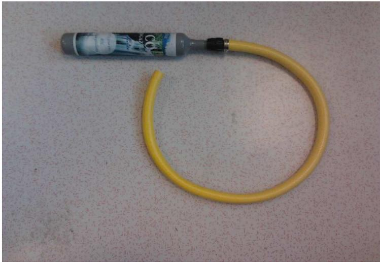
**Fig. xx: Carbon dioxide gas cylinder.** As compressed carbon dioxide is necessary in many activities, small cylinders similar to the one shown on the picture can be bought fairly easily and at low cost. The one represented here is used for the production of sparkling water, it weighs only one kilogramme and costs about 20 euros (10 euros for the empty bottle and 8 euros for a refill).
