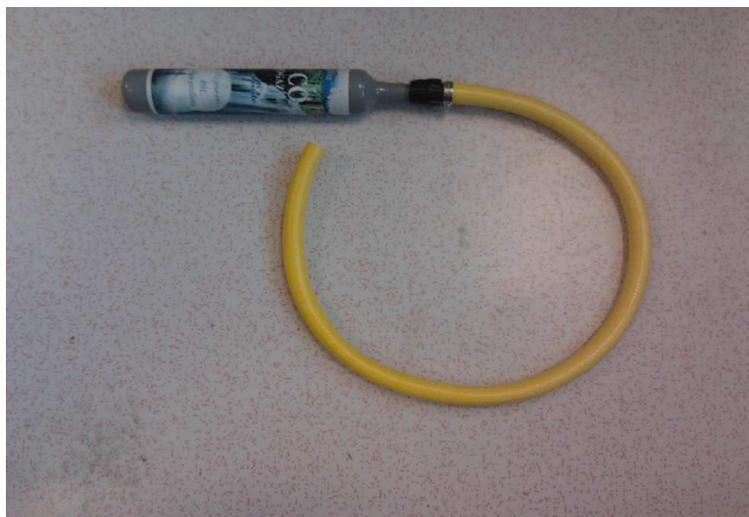
**Carbon dioxide gas cylinder.** As compressed carbon dioxide is necessary in many activities, small cylinders similar to the one shown on the picture can be bought fairly easily and at low cost. The one represented here is used for the production of sparkling water, it weighs only one kilogramme and costs about 20 euros (10 euros for the empty bottle and 8 euros for a refill).
